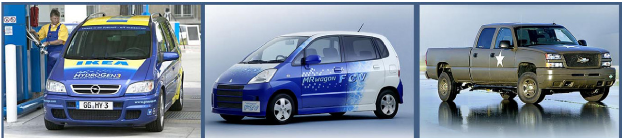
Fig. 10. The HydroGen3 system architecture (60 kW at the wheel) has been downscaled for integration into the Suzuki MR Wagon MR (38 kW at the wheel) and upscaled for propulsion of a Chevrolet Silverado military truck (120 kW at the wheel).
